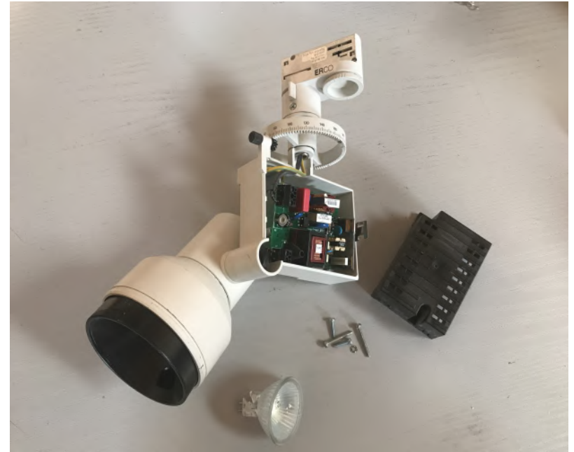
The tungsten halogen components in the fixture above are replaced by the optical LED assembly below.
